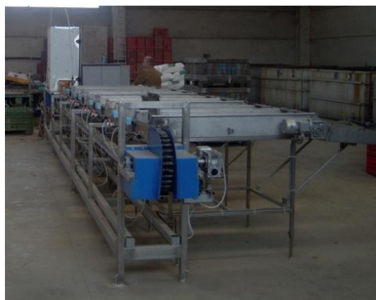
Figure 1. Overview of the machine. Featured tanks used to harvest cuttings according on the diameter class.
