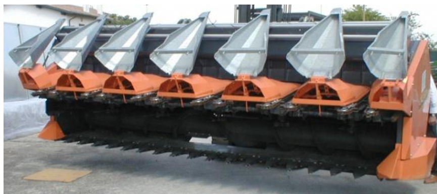
Figure 1. CRA-ING prototype built by Cressoni Firm: full-length mowing bar, in the low, and device operating on six-rows for stalks conditioning and detachment of the heads to be sent to the threshing system of the combine harvester, in the upper.
