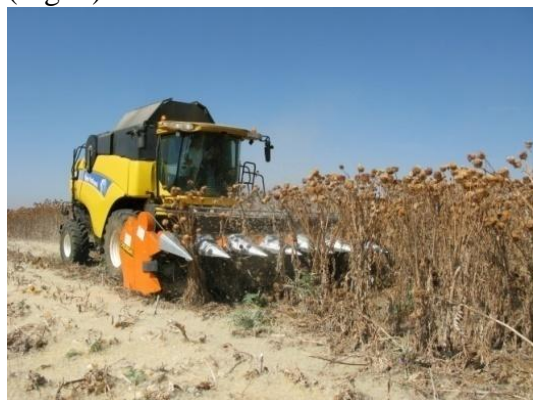
Figure 5. New Holland CX 8060 combine harvester equipped with Cressoni/CRA-ING Cynara Cardunculus head in harvesting phase
