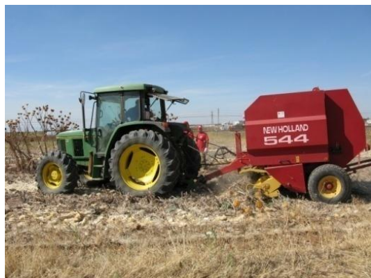
Figure 7. Harvesting and baling of the windrowed biomass by New Holland 544 roto-baler with fixed camera equipped with pick-up
