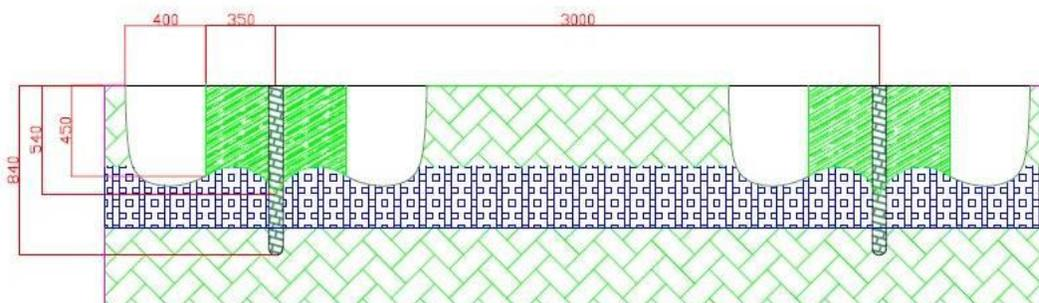
Figure 4. Scheme of vertical and central ripping of the soil
