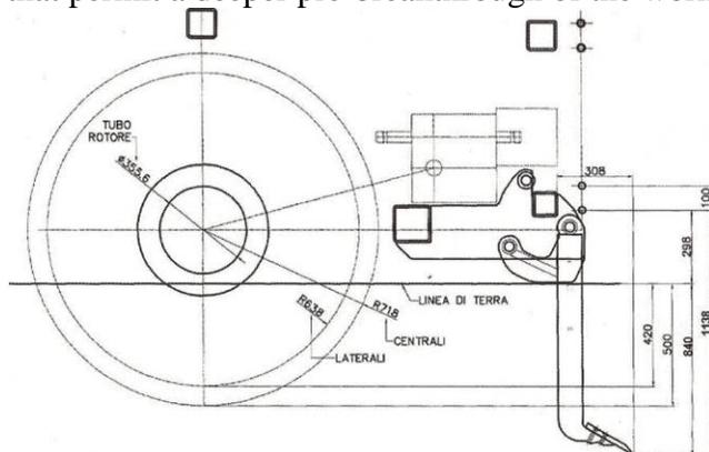
Figure 2. Diagram of the Falc rotative plow (model Falc Land 1500) modifications
