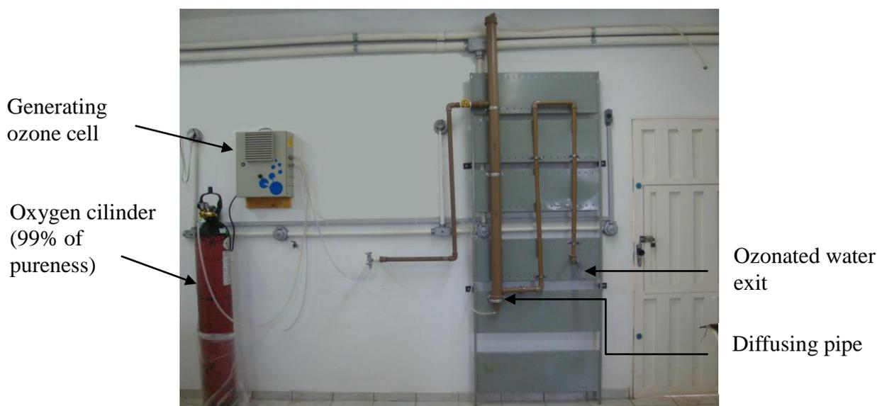
Figure 1. Equipment for production of ozonated water.
