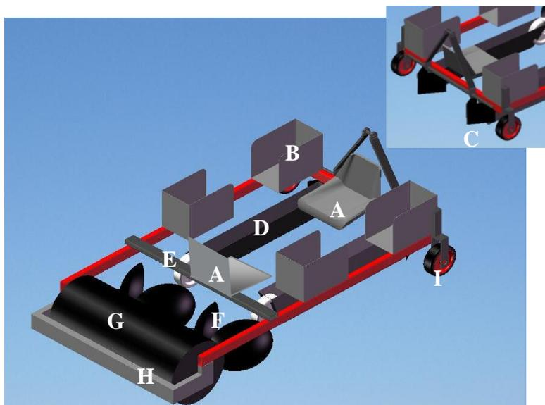
Figure 1. The prototype consists of: a) seat; b) lateral boxes for culms containing; c) “V” shake ploughs; d) metal structures avoid soil entering into the furrow; e) idle wheels hold culms back in the furrow; f) a couple of dual ridging discs serving to cover furrow; g) compaction roller; h) scratch-roller; i) idle wheels.
