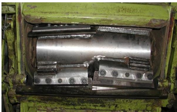
Figure 4. Ten fix knives as well slots to better fix the position on the knife holder are distinctly visible in the CRA-ING rotor
