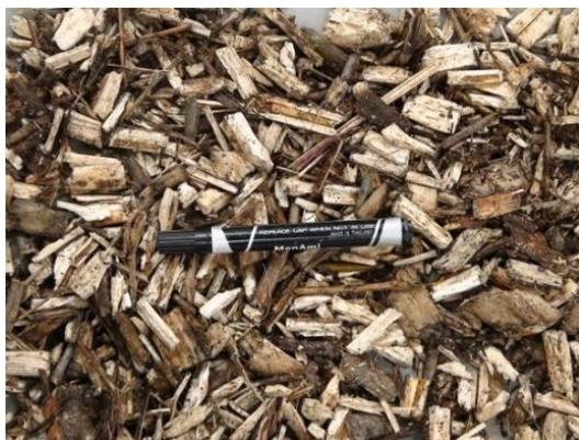
Figure 5b. Comparison of the chip obtained by Class Jaguar equipped with CRA-ING (a) and current rotor (b)
