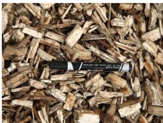
Figure 5a. Chip produced by CRA-ING rotor
