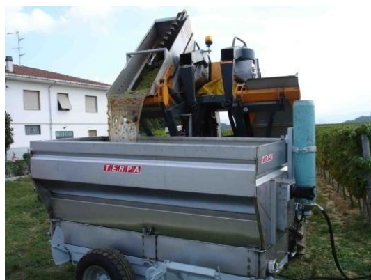
Figure 1. Grapes mechanically harvested and unloaded into the wagon modified for the must separation
