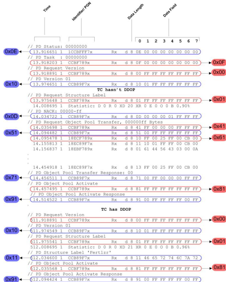
Figure 8. The CAN messages log of the initialization process among TC and WSM.
