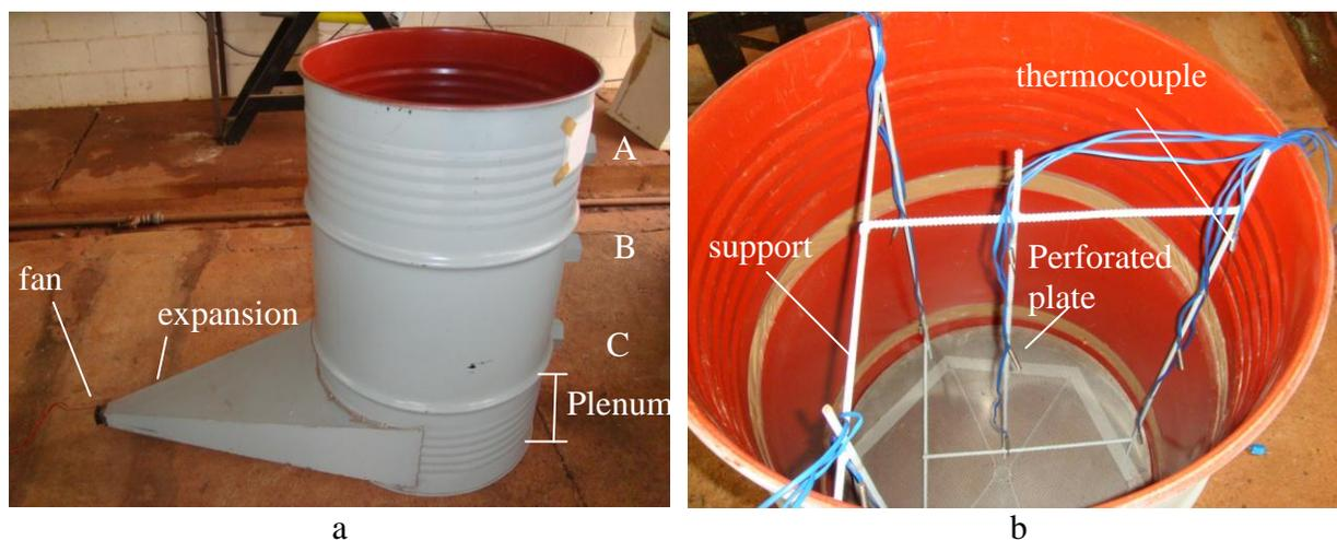
Figure 1. Exterior (a) and inside (b) of the bin with identification of its constituent parts.
