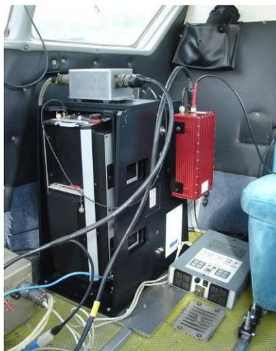
Figure 2. The installed spectral camera with red color OXTS RT3003 GPS/INS unit
